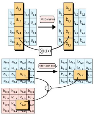
The block to be encrypted is just a sequence of 128 bits. AES works with byte quantities so we first convert the 128 bits into 16 bytes. We say "convert," but, in reality, it is almost certainly stored this way already. Operations in RSN/AES are performed on a two-dimensional byte array of four rows and four columns. Each round of the encryption process requires a series of steps to alter the state array. These steps involve four types of operations called:
